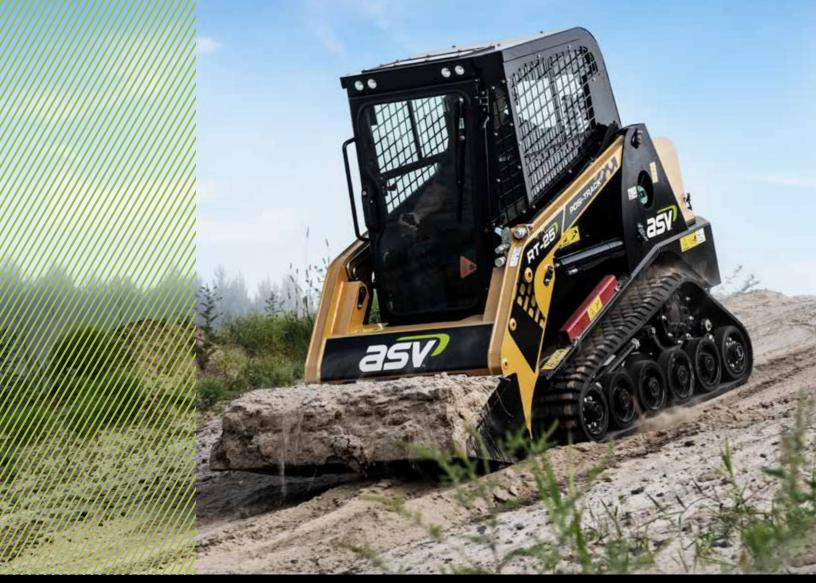
Introducing the all-new RT-25 Posi-Track® compact track loader—the smallest machine of its kind. The RT-25 features the productivity and comfort that landscapers, homeowners, rental centers, snow removal businesses, and contractors need. Designed small, the RT-25 offers patented Posi-Track technology with the suspension, traction, and flotation you count on to the shape the earth.
